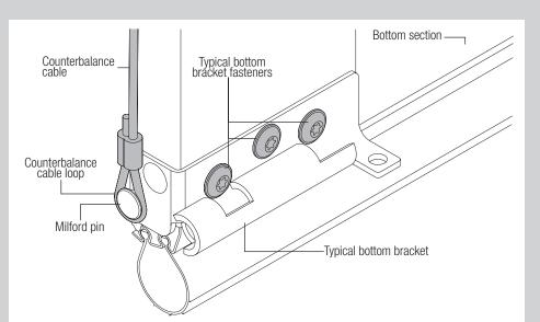
NEVER LOOSEN FASTENERS ON BOTTOM FIXTURE. USE CAUTION WHEN TIGHTENING FASTEN-ERS BECAUSE BOTTOM FIXTURE IS UNDER HIGH SPRING TENSION.
